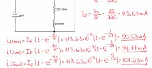
Q 47) For the circuit in the previous question, initially the final steady value of the current through the inductor is reached. Then SW1 opens and SW2 closes simultaneously. Determine the current through the inductor at 1ms, 3ms and 5 ms after the switch SW2 is closed. [3 marks]
