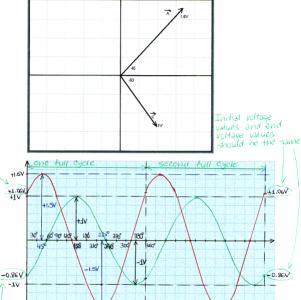
[V] At least one full cycle has to be clearly visible for each sine wave. Peaks and zero crossings should occur at their correct values. Amplitudes have to be proportional. Clearly label everything? Q 25) Determine the frequency for the angular velocity of 1256 rad/s
