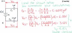
Q 31) What is the voltage between points A and B in the circuit below?
