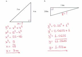
9. Determine the lengths X AND Y in the triangle below, using only trigonometry:
